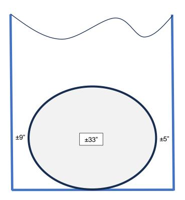
30-inch concrete inlet pipe on skew. Zero bottom clearance. Vault interior width ±48-inch.
