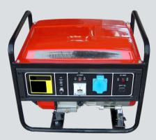
Typically, generators are run outside in open air and away from your house. This will ensure that the generator runs at the proper temperature and the exhaust does not enter your residence. Never refuel a generator while it is running or if the exhaust or engine is hot. Also, do not leave the generator running if no one is available to monitor its operation.
